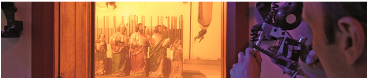
Figure 1 : Irradiation of polychrome wooden sculptures (Angels and Apostles, 17 th c., Le Pègue, France) for insect eradication.
