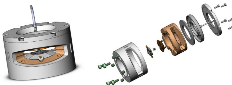
Figure 1: New Diamond Anvil Cell, mBX110, assembled and exploded view.
