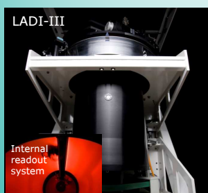
LADI-III: quasi-Laue neutron diffractometer
