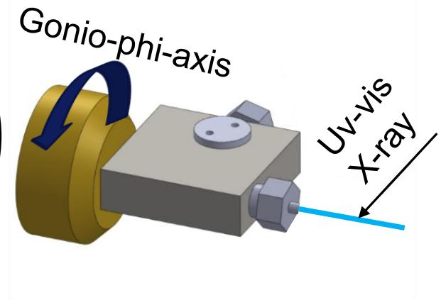
RT cell = microvalve 2kbar + capillary
