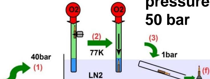
**Cryogenic O<sub>2</sub> pressure cell
