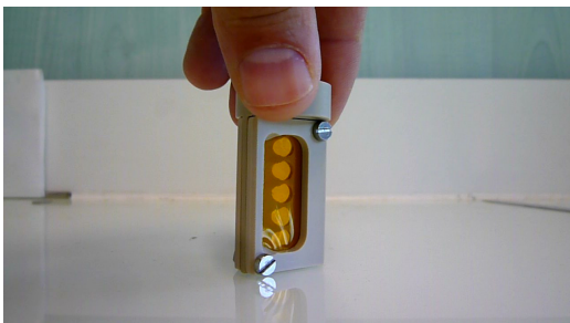
D.4 Left: back frame with the good orientation (samples are visible at 45°) Right: back frame with the wrong orientation (samples are masked at 45°)
