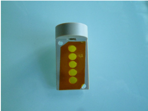
B.2 Remove the extra part of kapton that sticks out from the bottom, that covers the holes, etc.
