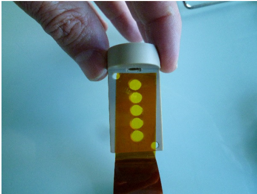
B.1 Put kapton tape on the analysis surface
