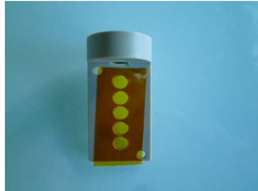
B.1 Put kapton tape on the analysis surface
