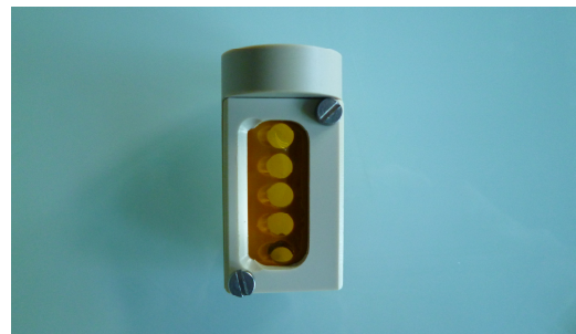
D.3 Flip the frame back and position it on the holder by inserting the two bolts. Be aware that the frame is asymmetric, and only one position is possible!
