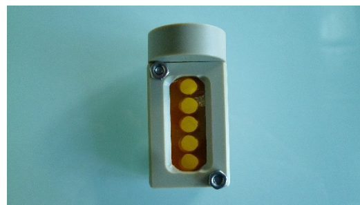
D.6 Position the Analysis surface frame (A.4) and the corresponding nuts. Screw them, not too tight (the frames and holder are fragile)
