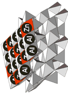
Figure 3. Proposed crystallochemical environment for Zn uptake on Al-mont, as inferred from EXAFS results.
