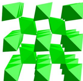
Figure 4. Schematic drawing of the tetragonal crystal structure of \beta - \text{MnO}_2 viewed along [001] .
