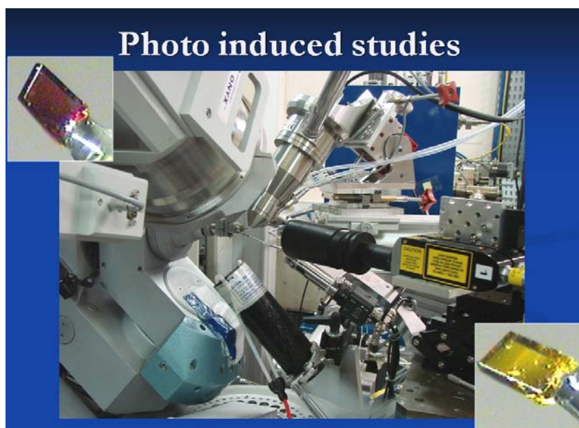
Figure III.4. Example of an in-situ experiment carried out on the KM6 diffractometer
