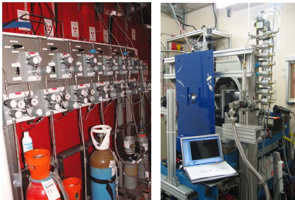
Figure III.10. The array of gas bottles outside the experiment hutches, and the gas mixing system designed for high gas pressures installed on the MAR345 image plate setup
